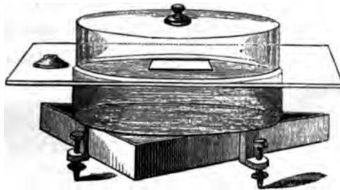
FIG. 8.—APPARATUS EMPLOYED FOR PLATE-CULTIVATIONS. Tripod Stand; Glass Dish, filled with cold or iced water; Sheet of Plate-glass; Spirit Level, and Glass Bell.
